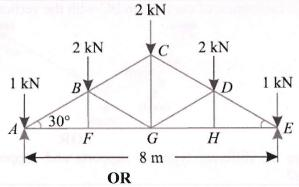
8 Determine the nature and magnitude of the forces in the members BC, GC and GF of the truss shown in figure?
